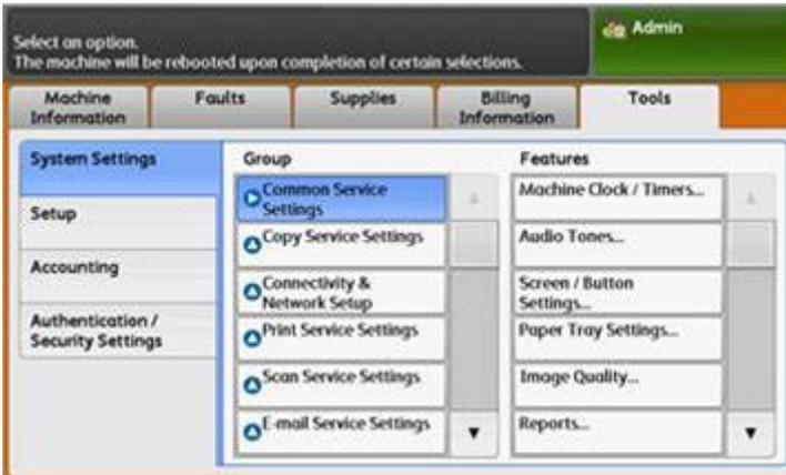
4. Select **System Settings->Common Service Settings** and scroll down on the **Features** column to access the **Other Settings** screen.
