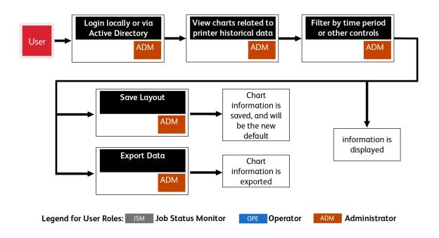
Figure 2.4 Xerox® FreeFlow® Vision Workflow – Manage Administrator Tasks
